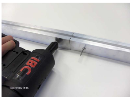
Illustration 24: Riveting the rails with butt connectors
