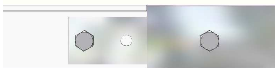
Fig. 36: Butt connector for aluminum L-section 60x40x5 roof hook connector
