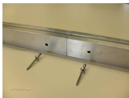
Illustration 23: Drilling the rails with ø4.9mm drill bit for 2 dome head blind rivets 4.8x10mm
