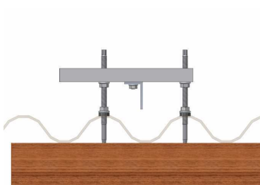
Fig 13.1: Correctly fitted hanger bolt with aluminum L-section roof hook connector
