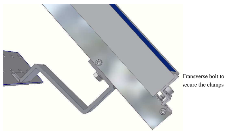
Fig. 28: Clamps secured against slippage
